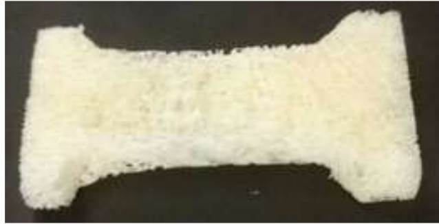
Figure 5.3. The machined demineralized bone graft prepared for tensile test.
