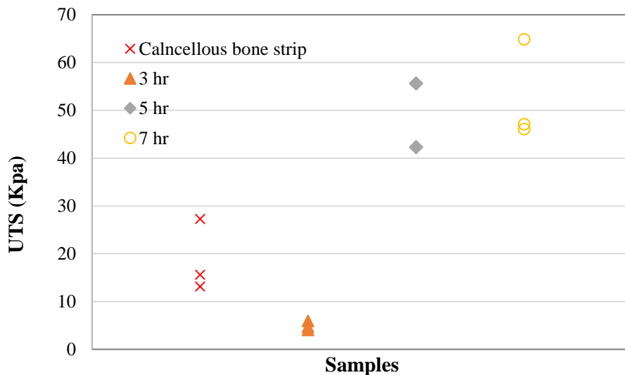
Figure 6.14. The comparison of the maximum tensile strength of the heat treated samples to the natural cancellous bone strips.
