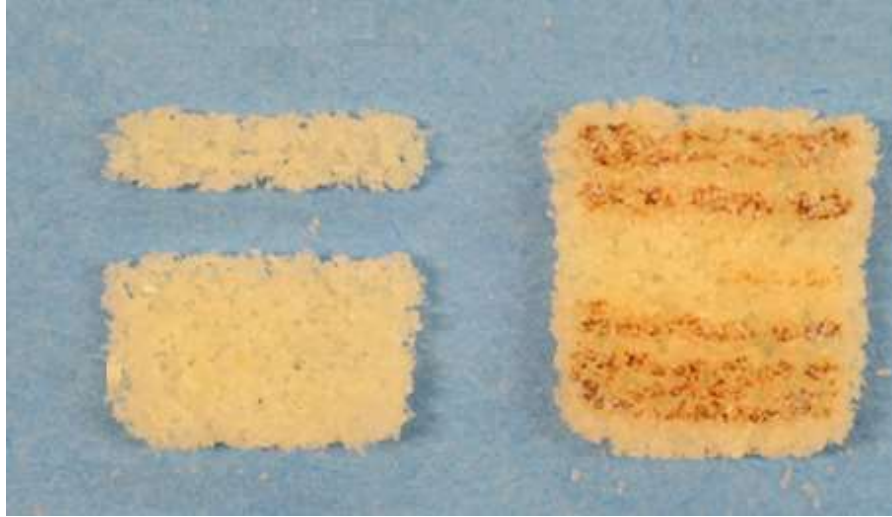
Figure 6.6. An example of laser fluctuation effect at scanning speed of 50 mm/s or 100 mm/s. Left: incomplete layer at lower bound, Right: Discolored bone traces at upper bound.
